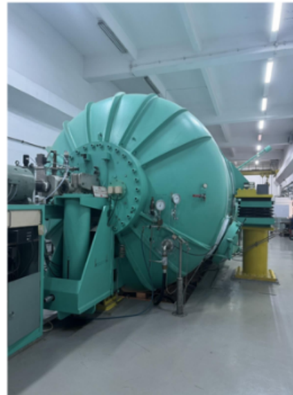
Fig 1: The 9 MV Tandem accelerator in IFIN-HH
